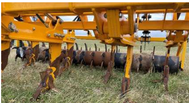
Image 1. A 3.15m wide TARIM OZ 9 leg Hydropneumatic Subsoiler with spiked packer rollers was used to incorporate clay.
