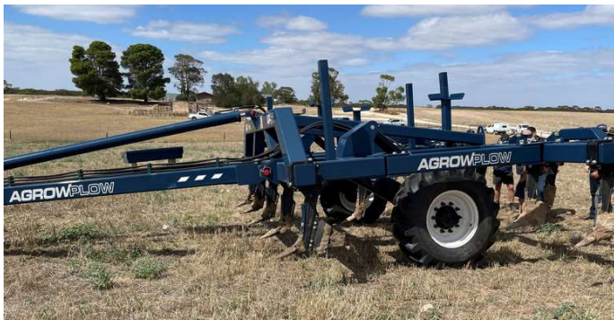
Image 1. Agrowplow Deep Ripper with inclusion plates fitted on the outside shanks.
